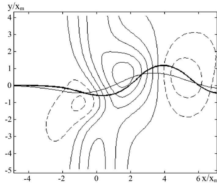
**F i g. 2.** The mid-jet path (thick line) superimposed by the stream function in the lower layer (dash lines show positive (anticyclonic) deep eddies) of the two-layer model for  $t = 2x_m/v_m$ ; solution (11) – (13) is shown by a thin line
