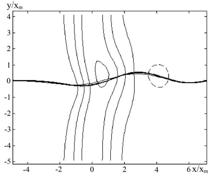
**F i g. 1.** The mid-jet path (thick line) superimposed by the stream function in the lower layer (dash line shows positive (anticyclonic) deep eddies) of the two-layer model for  $t = x_m/v_m$ ; solution (11) – (13) is shown by a thin line
